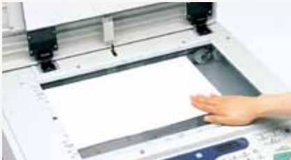
1. Set the original and press the start key to make a master.
